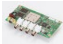
Video Input Unit NS-CA001 • NTSC/PAL video inputs (4 channels)
